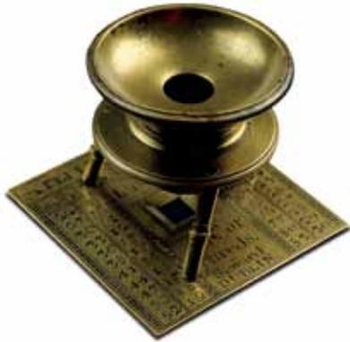
Linen prover, Seward, Dublin, mid-18th century. Magnifier used for measuring the density of threads in linen cloth for the purpose of quality control
