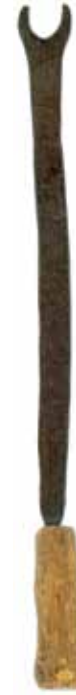
A spurtle (a small fork) from Clones, Co. Monaghan used in thrust thatching to knot small bundles of straw into place
